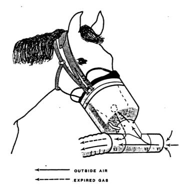
Figure 2. Face-mask used with respiration calorimeter.
