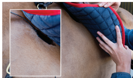
The upper sensor rests under the saddle, and its position is maintained through the pressure of the saddle. A second sensor is placed under the girth.
