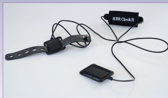
KER ClockIt Sport includes a small transmitter and two thin sensors. One sensor is positioned under the saddle and another under the girth.
